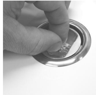
Step 3. Grip the halogen bulb and pull from holder
